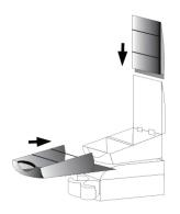
**Step 1.** Slide on console top, then console bottom.
