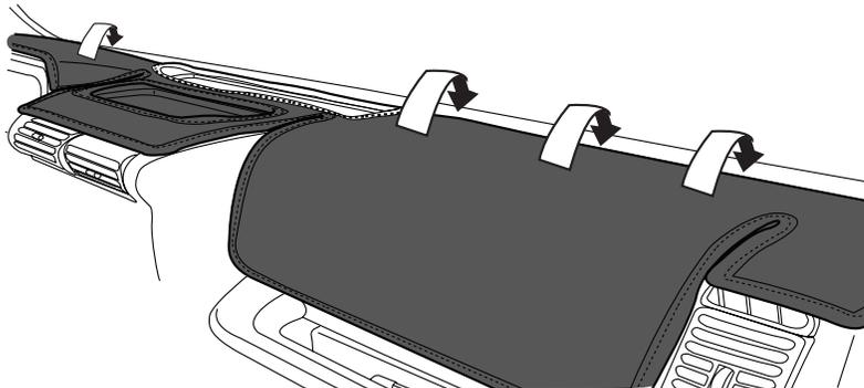
**TIP:** Because of auto assembly tolerances or variations in the position of replacement windshields, dash covers may require trimming on the windshield edge.
