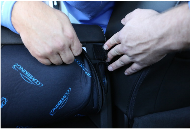
Adjust the seat back along the console lid and tighten the upper Velcro strip
