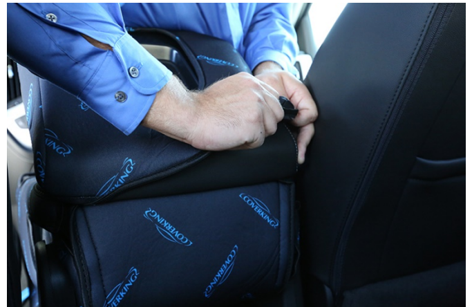
Tuck the back of the console cover over the rear corners of the top console
